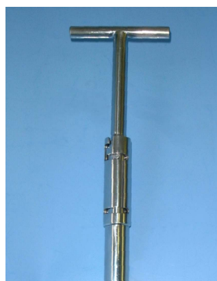
Bayonet fitting allows two samples to be taken at the same sampling point
